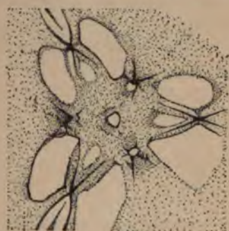
FIG. 11. — "Light figure" seen upon an etched surface of a crystal of calcite (after Goldschmidt and Wright).
